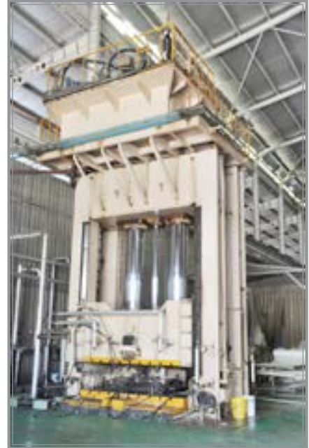
State-of-the-art 600 metric tonnes hydraulic press, one of the country's biggest units for FRP water tank panel moulding.
