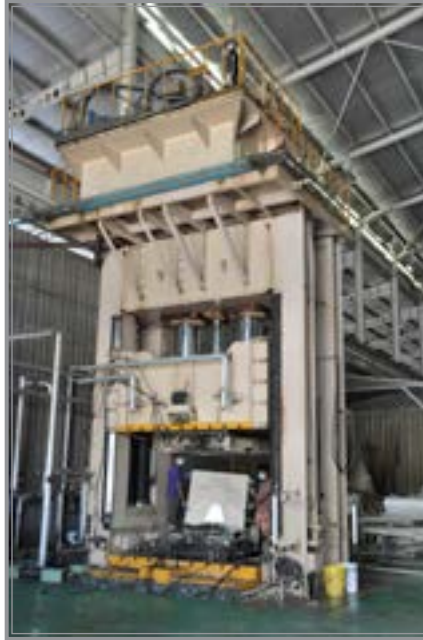
State-of-the-art 600 metric tonnes hydraulic press, one of the country's biggest units for FRP water tank panel moulding.
